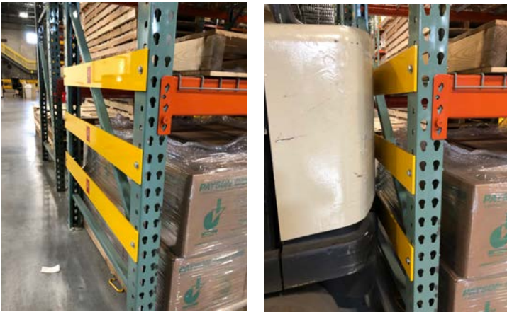
Reinforces rack and protects from impact
