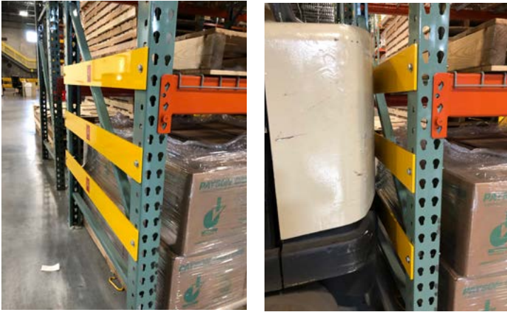
Reinforces rack and protects from impact
